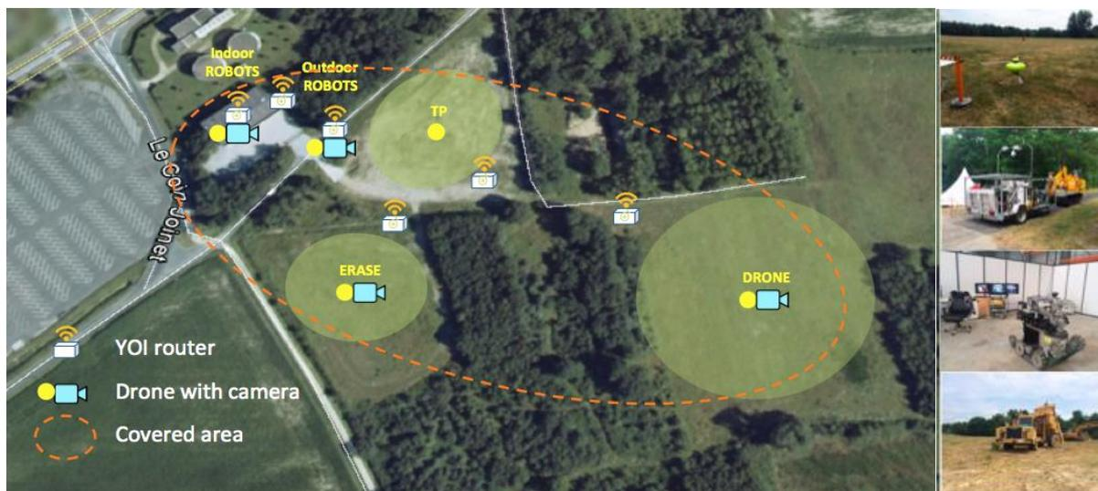
Once the network turned on, rescuers could access real time videos and embedded services such as a chat and VoIP application by using a regular smartphone, a tablet or a laptop connected to the secure Wi-Fi. **All services and security were previously embedded and distributed into the network without any single point of failure** in order to provide the rescue with maximum of autonomy, interoperability and mobility.
